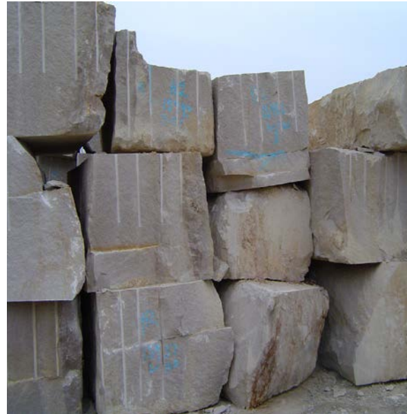
An existing old quarry cut in the limestone bluffs of the Ohio River, near the proposed bridge landing, indicates the St. Louis layer of limestone that would be revealed in several corridor road cuts.
