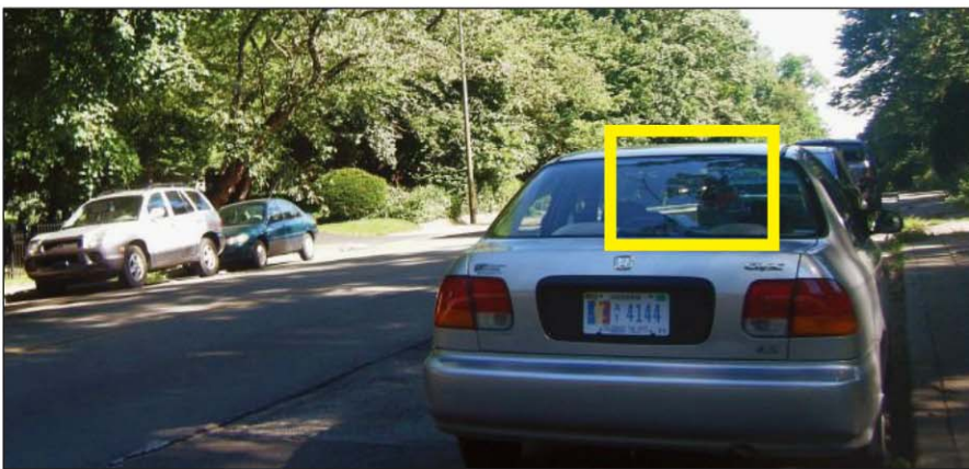
Figure 2. Position 2—car at just under 300 ft. (92 m) from intersection, beginning to be visible through the windshield of the parked car.
